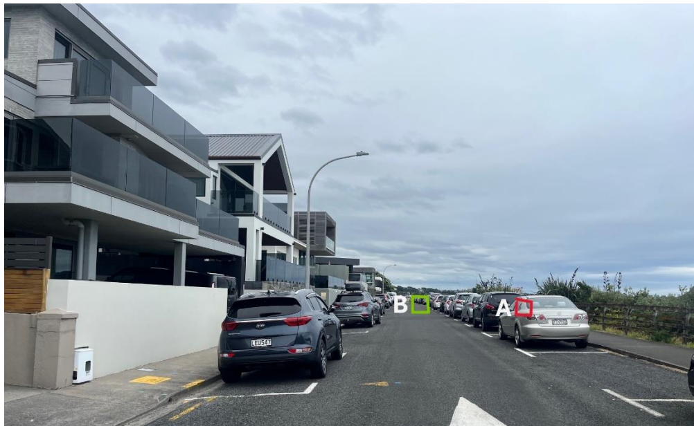
Approximate location of nail datum (A) on footpath and survey level 17.18m (B) on roadway
