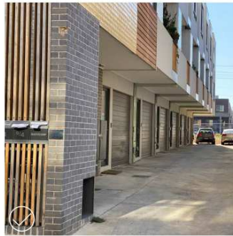
Locating car parking along a side laneway reduces the vehicular impact on the street.
