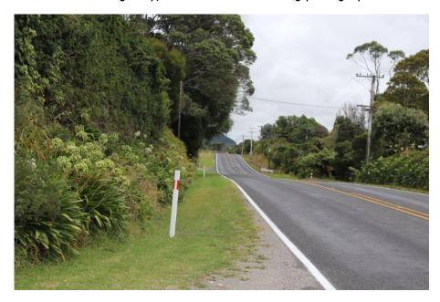
Whilst the road surface disappears past the crest curve following the culvert, vehicles remain visible for the full sight distance as demonstrated in the following photograph:
