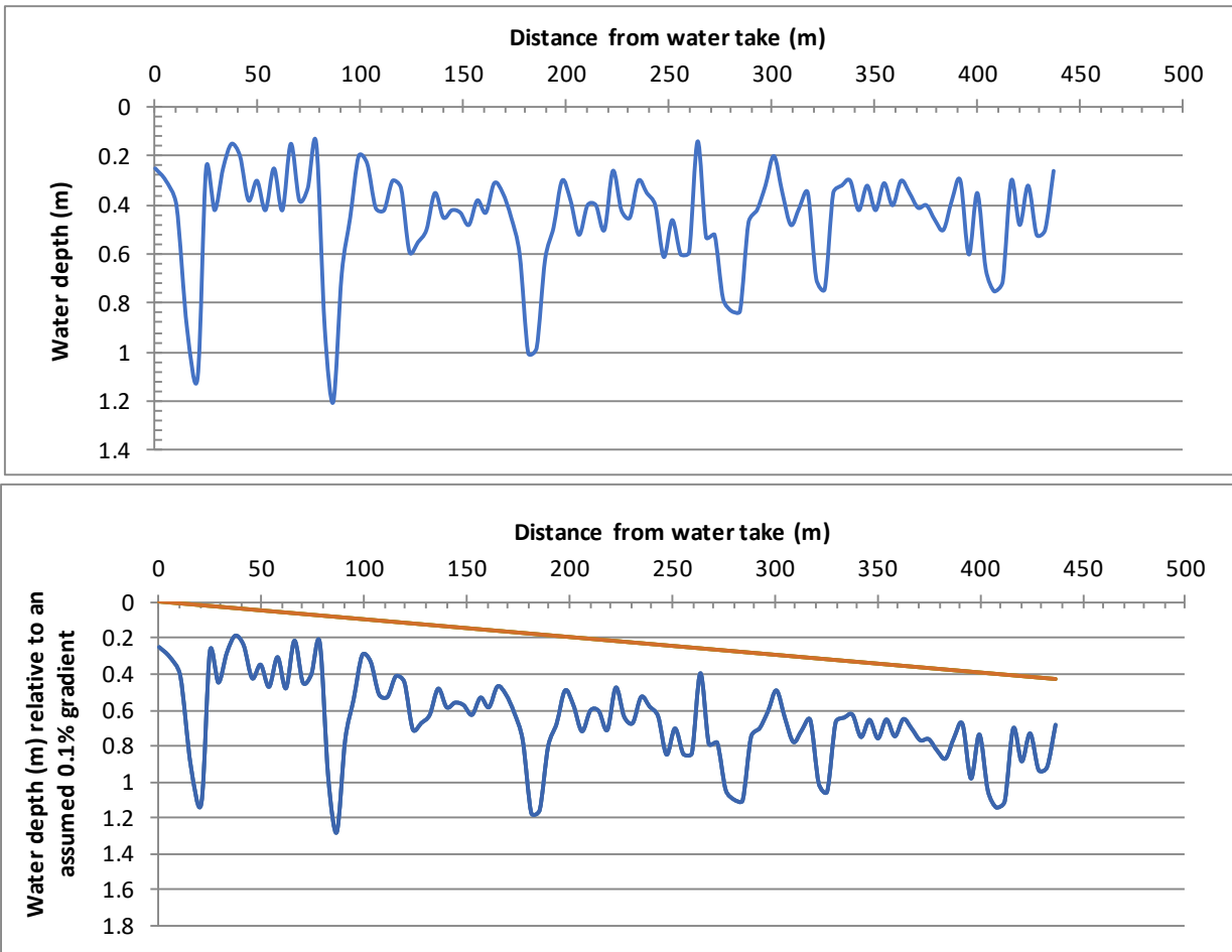
Figure 2.2 – Water depth longitudinally down the Mangapepeke Stream, downstream of the proposed water take (1 November 2017). The top graph is relative to water level, the bottom graph has an assumed gradient of 0.1%.
