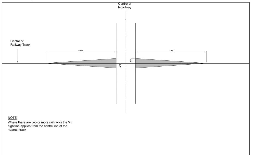
Diagram 19.2 Railway level crossing sightline distances at controlled crossing with 70km/h maximum railway line speed
