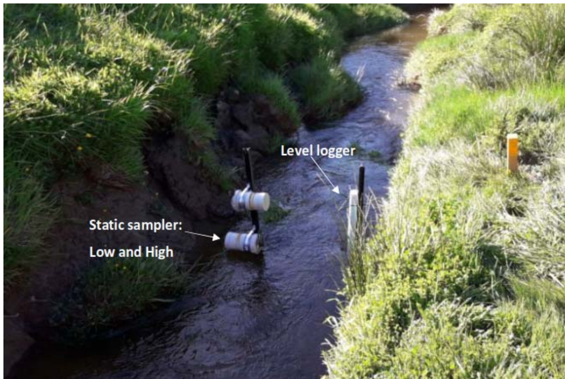
Figure 4.1 – Static sampler and level logger configuration at WQ4
