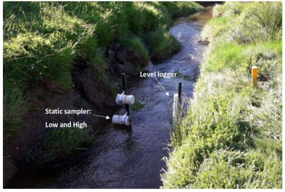
Figure 3.2: Static sampler and level logger configuration at WQ4
